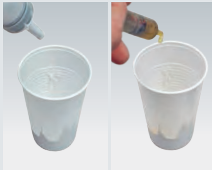
2] Dosage: Epoxy resin: 6 parts (ml) Epoxy hardener: 1 part (ml) ...
