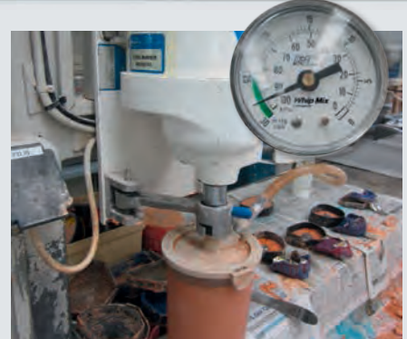
9] SAE special die stone mixed in the vacuum mixer – 1 minute at 15-20 millibar.
