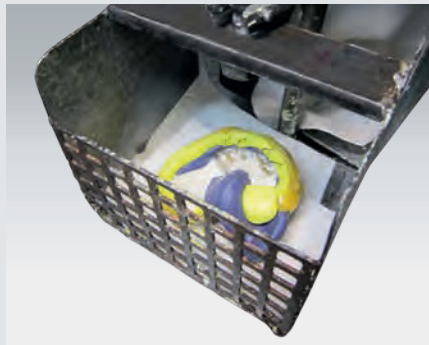
5] Position impression in the horizontal centrifuge with counterbalance. Spinning process: 1 minute
